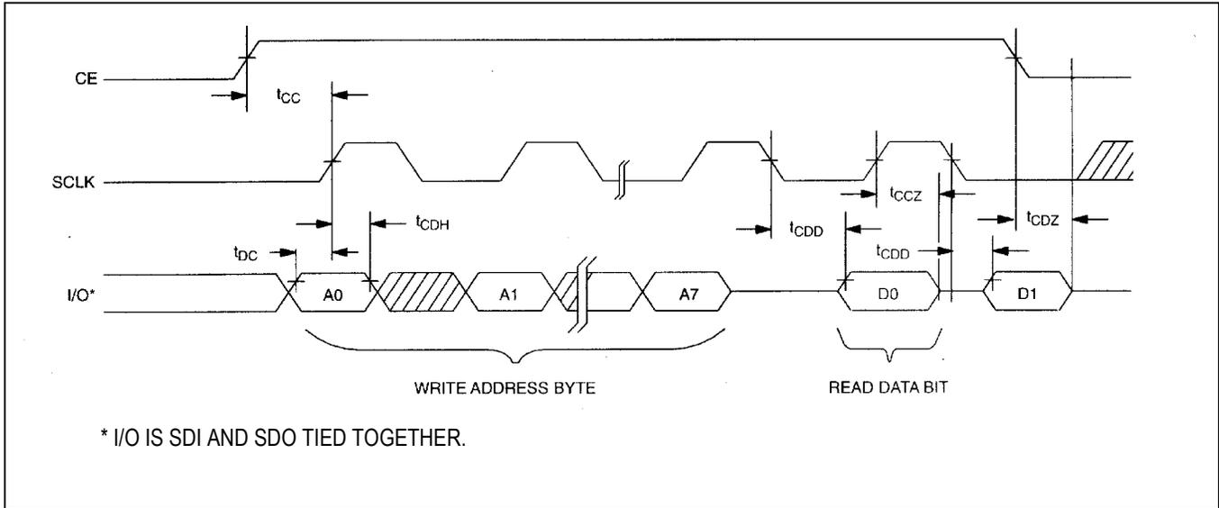
**Figure 11. TIMING DIAGRAM: 3-WIRE WRITE DATA TRANSFER**
