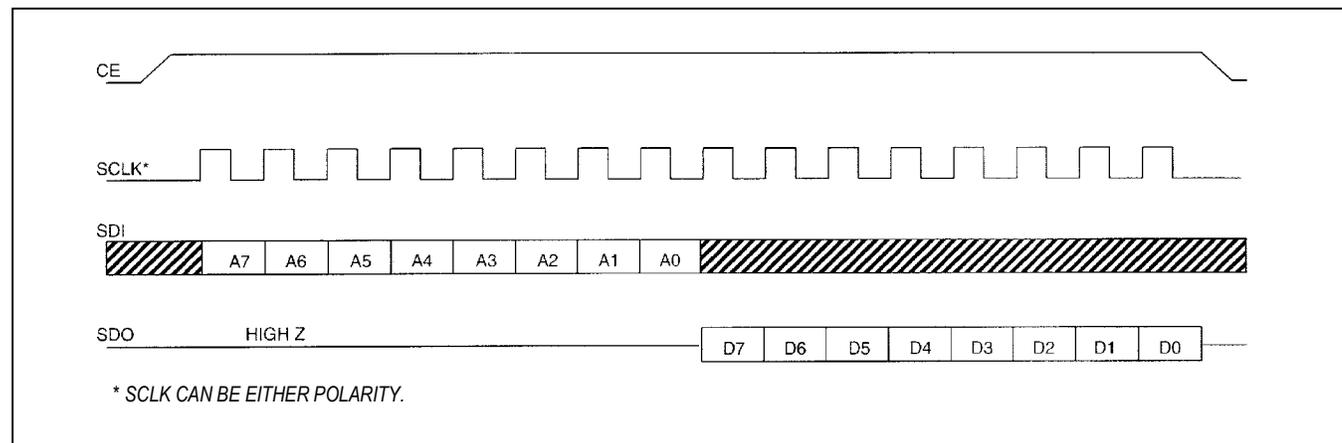
The address byte is always the first byte entered after CE is driven high. The most significant bit (A7) of this byte determines if a read or write takes place. If A7 is 0, one or more read cycles occur. If A7 is 1, one or more write cycles occur.
