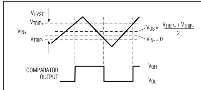
Figure 1. Input and Output Waveforms, Noninverting Input Varied
