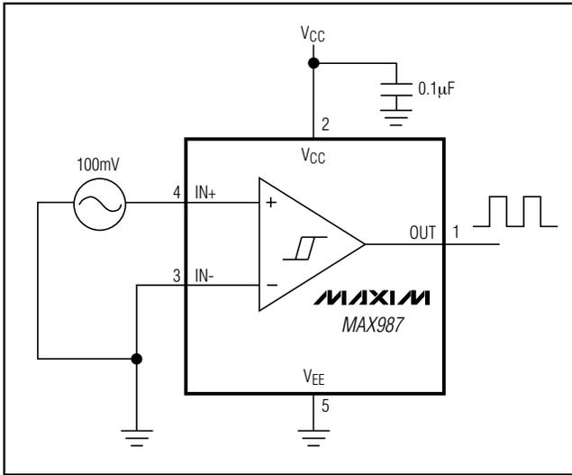
Figure 3. Zero-Crossing Detector
