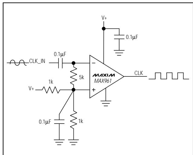
Figure 6. Clock Generation Circuit Using Low-Noise Comparator
