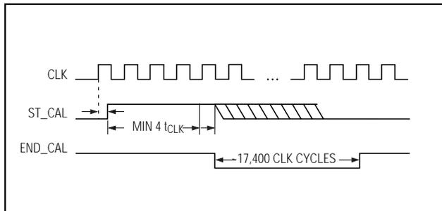
Figure 8. Timing for Start and End of Calibration
