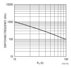
Figure 4. Switching Frequency vs R<sub>T</sub>
