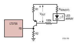
Figure 3. Feedback Resistor Connection for Buck Mode or Buck-Boost Mode LED Driver
