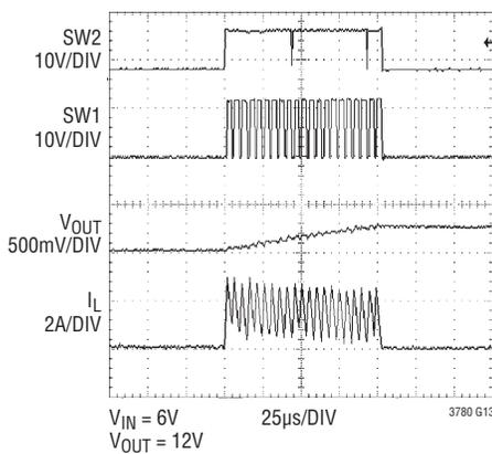
**Burst Mode Operation ( $V_{IN} = 12\text{V}$ ,  $V_{OUT} = 12\text{V}$ )**
