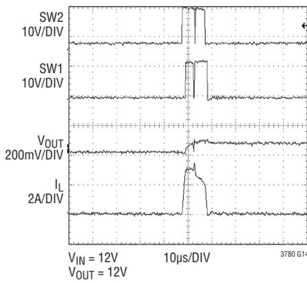
**Skip-Cycle Mode ( $V_{IN} = 18\text{V}$ ,  $V_{OUT} = 12\text{V}$ )**
