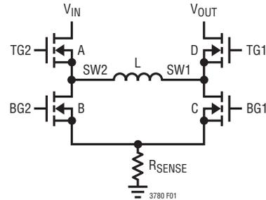
Figure 1. Simplified Diagram of the Output Switches
