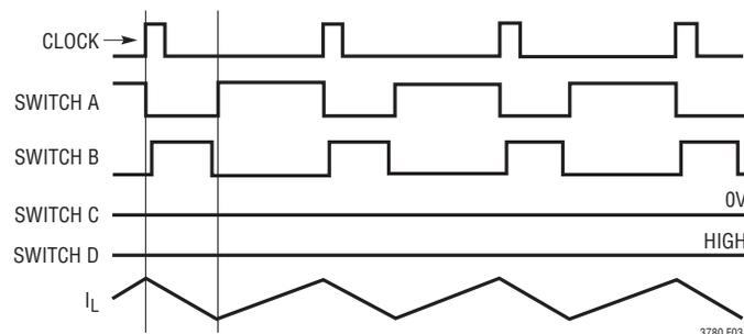
Figure 3. Buck Mode ( $V_{IN} > V_{OUT}$ )
