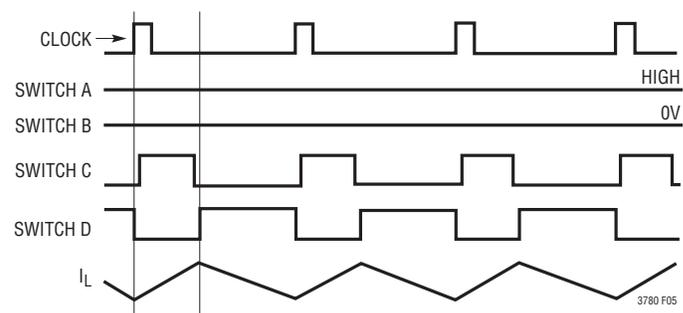
Figure 5. Boost Mode ( $V_{IN} < V_{OUT}$ )
