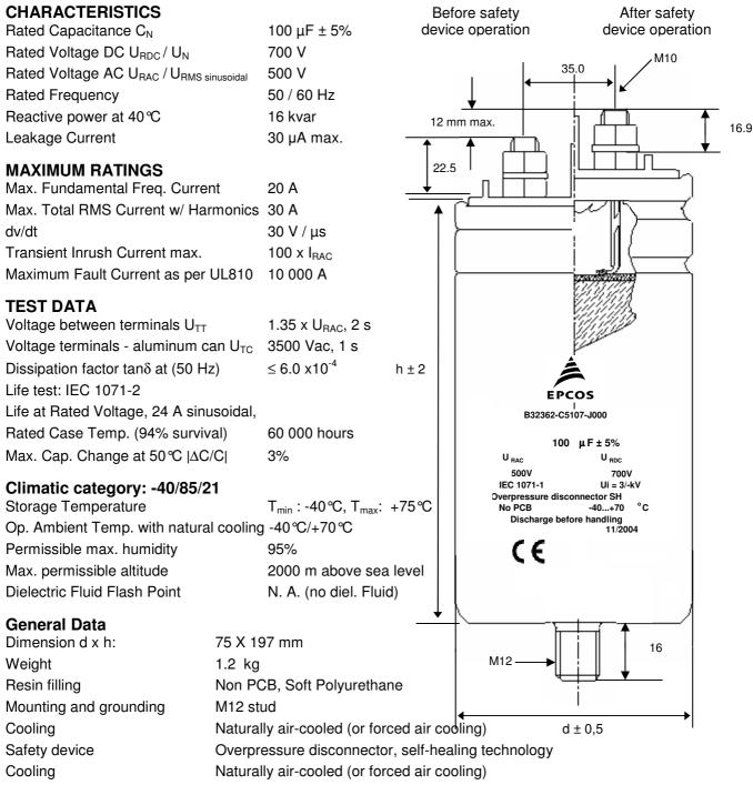
Degree of protection Indoor mounting **Terminals** M10 screws IEC 1071 Reference standards
